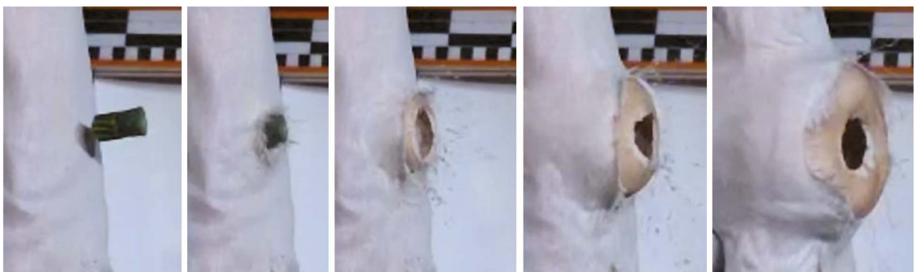
Fig. 4. Frame-by-frame reproduction of the target hit process by the UNO 35E cartridge slug.
