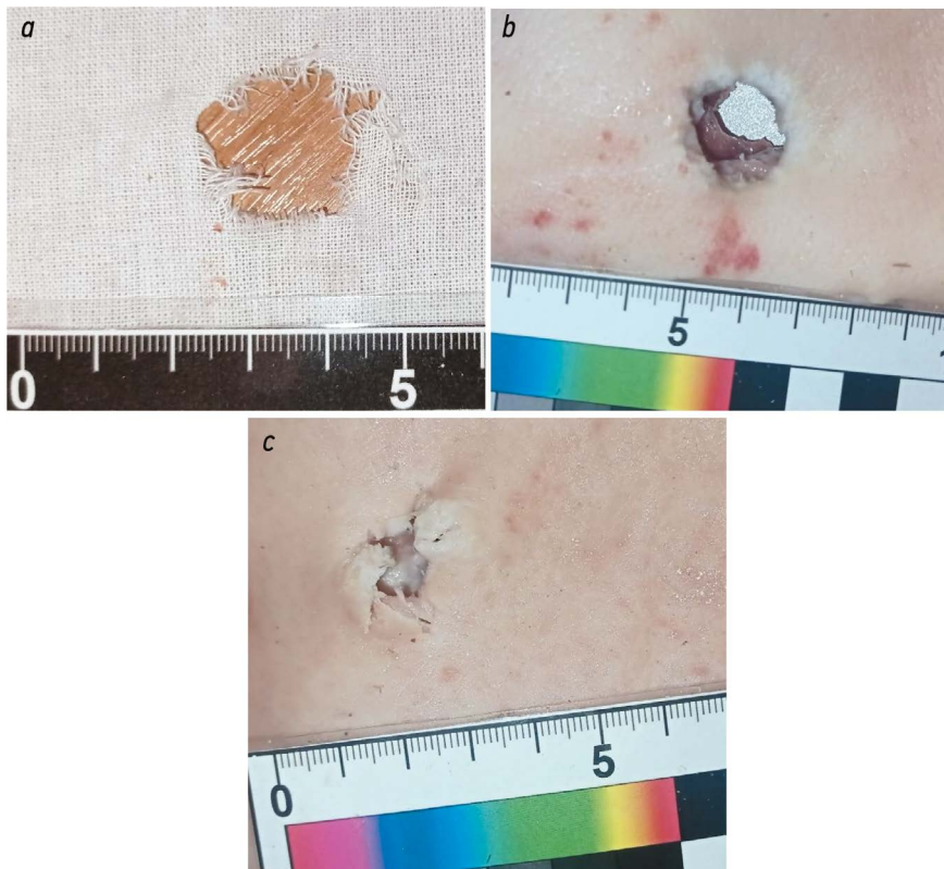
Fig. 2. Experimental gunshot damage after firing UNO 35 cartridge: a — on cotton fabric; b — an entrance gunshot hole at biological simulator skin; c — an exit gunshot hole at biological simulator skin.
